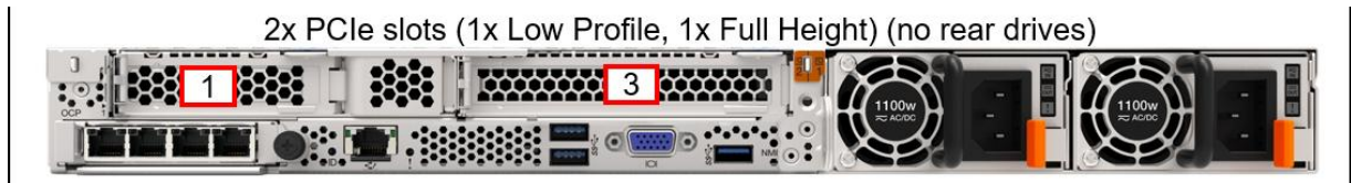
Figure 12: Rear view of the ThinkSystem SR645 V3 with 2 PCIe slots
